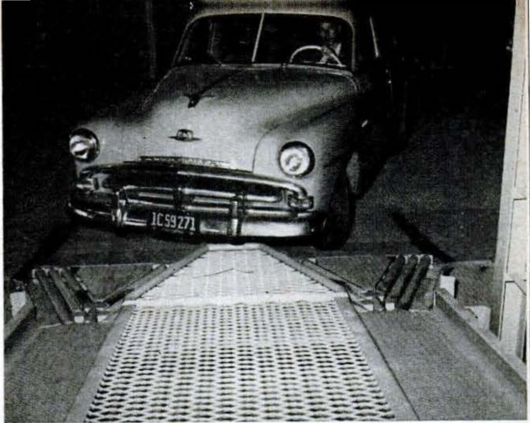
CARS ARE "FUNNELED" into narrow trackways of ramps and parking stalls by converging curbs. Rollers let wheels slip sideways.
